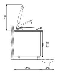
CWI1 Cold Water inlet 1 (cleaning) Electrical inlet (power) ΕI Hot water inlet
